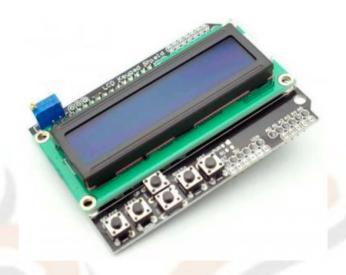
This is a very popular LCD Keypad shield for Arduino or Freeduino board. It includes a 2x16 LCD display and 6 momentary push buttons. Pins 4, 5, 6, 7, 8, 9 and 10 are used to interface with the LCD. Analog Pin 0 is used to read the push buttons. The LCD shield supports contrast adjustment and backlit on/off functions. It also expands analog pins for easy analog sensor reading and display.
